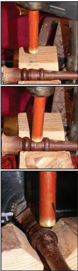
Above: Making ornamental cuts with a 1/2" diameter brass tube.
