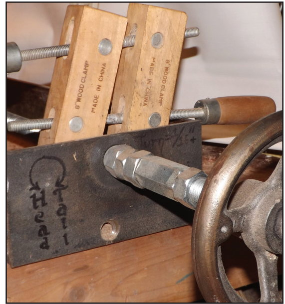
Above: A Jorgenson clamp works well to lock the spindle, keeping the crank in place.
